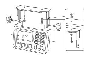
• **DASHBOARD MOUNTING** (with optional MB-75): For mounting the DS-100 to a dashboard panel.
