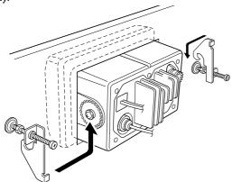
④ Tighten the end bolts on the clamps (rotate clockwise) so that the clamps press firmly against the inside of the instrument control panel.
